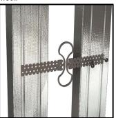
Connect the acoustic wall tie from the nail plate to the first vertical stud using in minimum two suitable fixing screws. Below picture shows installation examples for steel profile and veneer lumber studs.
