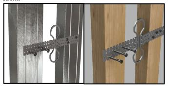
4. Cut the extra nail plate part out or bend it as shown in below picture example.
